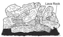
Figure 26 - Installing Lava Rock
